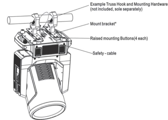
Fit bracket's keyed hole and locking mechanism over raised mounting buttons and slide forward.
