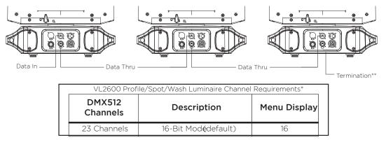
\*\*DMX terminator required for last fixture on DMX line.
