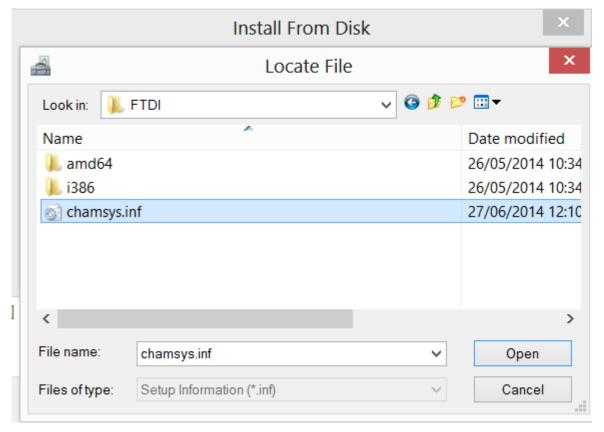
If the MagicQ USB wing periodically disconnects and restarts then check the Windows settings for your USB ports - Windows may be shutting down the USB ports when it incorrectly thinks they are idle. Click on Control Panel, System, Device Manager
