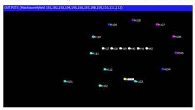
The movement view shows the relative positions of heads in terms of pan and tilt range on a 2D map. It also shows the current colour of the heads. This enables previewing of FX and relative positions without the lighting rig. Press the VIEW CHANS, VIEW DMX, VIEW MOVE soft buttons.
