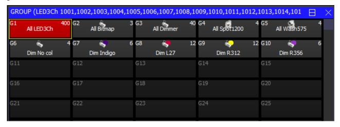
Using the auto groups, it is then possible to use standard FX such as RGB, sine waves, pulses to generate FX on your grid.
