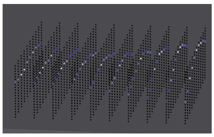
This effect takes the input media from it's own layer, and uses Modulate Layer 1 to offset the vertical position of the layer in 3D space and the Modulate Layer 2 to change the amount of blur. The vertical position and blur are calculated per column, so wave effects can be applied by using the "Organic" 2D FX on the Modulate 1 layer.
