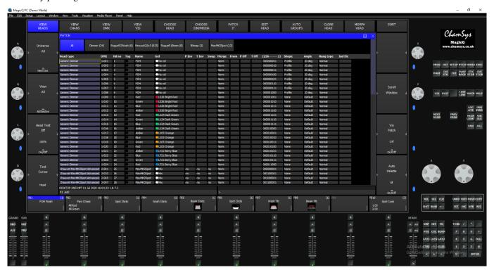
You can also test channels by moving to the appropriate channel and pressing the TEST SELECT CHANS soft button. The channel will be set to the level of the Grand Master fader. Pressing TEST SELECT CHANS soft button again returns the channel to zero. You can test multiple channels by using SHIFT and the cursor keys to select multiple channels and then pressing the TEST SELECT CHANS soft button. Channels that are in test mode are highlighted in red.
