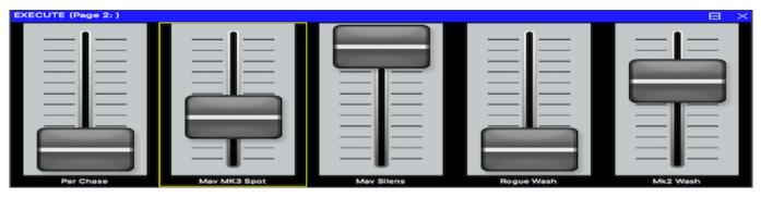
From version 1.8.8.0 MagicQ supports full sizing of all Execute items using the Item Width and Item Height soft buttons and encoders. In previous versions, and in 1.8.8.0 if faders are set to width and height of 1 then the size faders then if there is an unused box below the fader item then MagicQ automatically adjusts in the Execute View to fill the two boxes.
