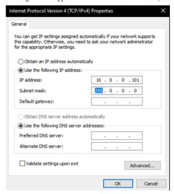
Choose "Use the following IP address". Enter the *IP address* (e.g. 2.0.0.10) and the *Subnet mask* (e.g. 255.0.0.0). The default gateway can usually be left blank. Click **Ok** then **Ok**.
