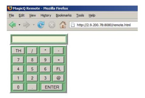
In order to set up a PC, Pocket PC or mobile phone to connect to MagicQ you must ensure that there is a physical connection to MagicQ – either directly via network cable, or via a wireless router. The IP address of the PC, Pocket PC, or mobile phone must be set to be on the same network as the MagicQ – this is generally the Art-Net IP addressing scheme – so the device must have an IP address starting with 2 (e.g. 2.0.0.2) and a subnet mask of 255.0.0.0.
