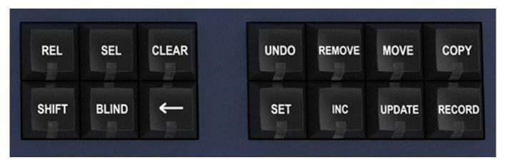
The Editor buttons are used to modify program data. The 8 buttons on the right hand side are the action buttons which are used to modify show data. The action buttons are UNDO, REMOVE, MOVE, COPY, SET, INCLUDE, UPDATE, and RECORD.
