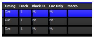
As a Cue Stack is executed, it keeps track of channels that have been used in previous Cues but are not used in the current Cue. How these channels are handled depends on the following settings on each Cue in the Cue Stack – there are three options which are shown in the Track field.
