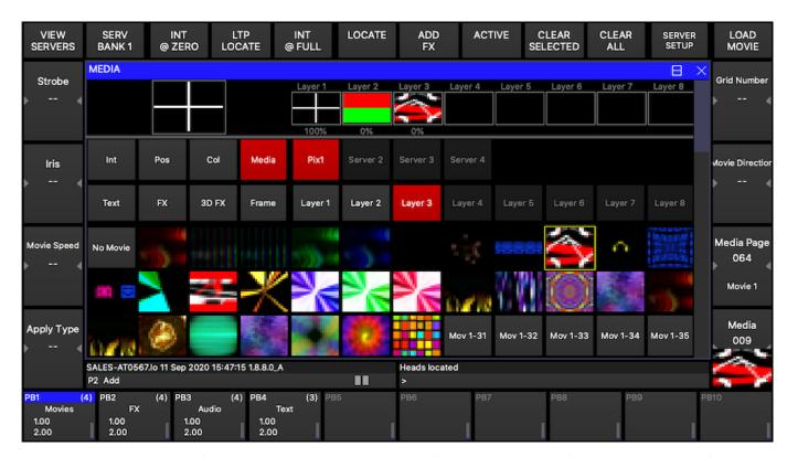
MagicQ asks the user to specify the number of layers required and will patch that number of layers (generic bitmapfx2 heads). The layers will be named according to the grid that is selected in the Outputs Window. MagicQ uses head numbers above the other patched heads.
