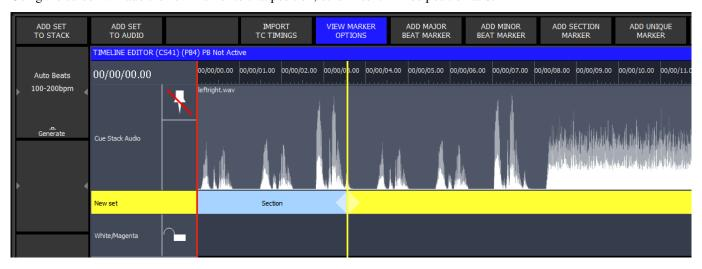
To add a new marker set layer you need press either the "ADD SET TO STACK" or "ADD SET TO AUDIO" option. The latter of the two options will only appear if there is and audio file assigned to the cue stack.
