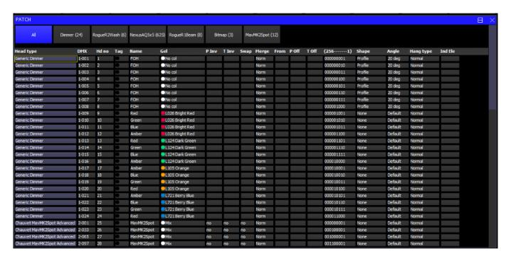
The gel field uses gel numbers. For Lee colours enter the gel number directly (e.g. 181 for Lee 181). For Rosco colours enter the gel number preceded by a dot (e.g. .14 for Rosco 14). For no colour enter 0. If you would prefer to use colour names rather than gel numbers then simply enter the colour name.
