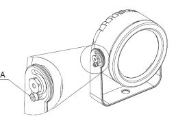
The screw must be fastened by using a 3 mm (0.118 in) hex key, not included.
