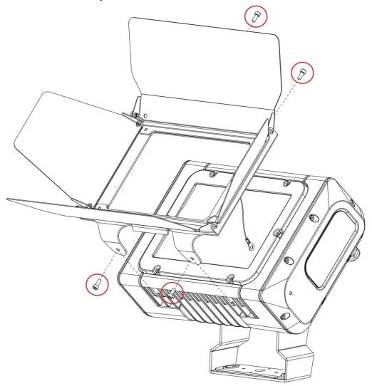
Once installed, fix the safety cable on the side cap by using the marked screw and the washer provided in the box as shown in the picture.
