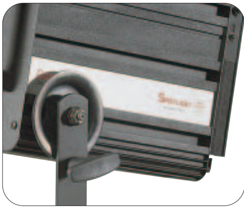
Reversible yoke mounted onto extruded sliding rails, adjustable height for correct balancing of the accessories and for use in any position
