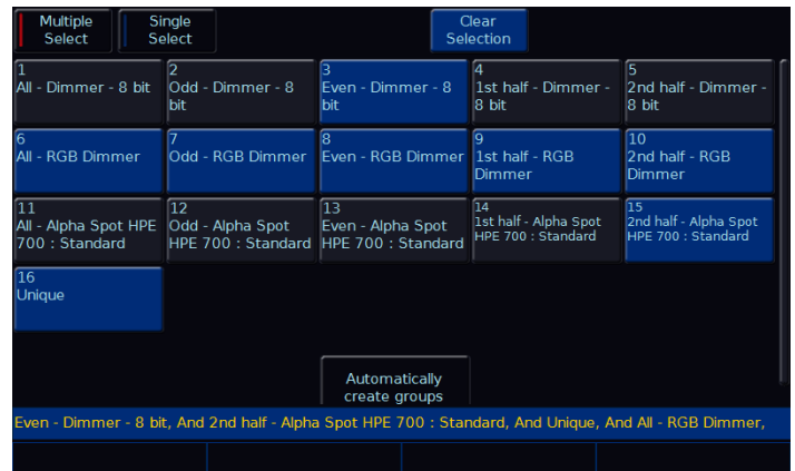
Groups window with various fixtures current selected highlighted in blue
